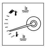
This gage shows the engine coolant temperature.
